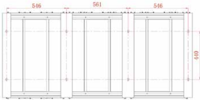
Figure 1.2 IES-R18 Rack fixed hole size drawing (unit: mm)
